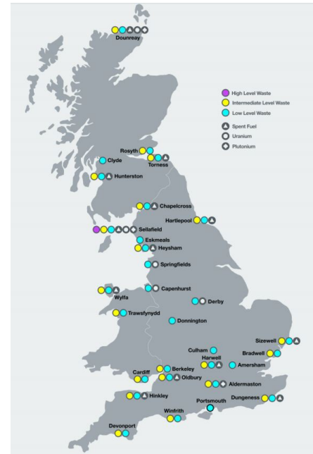
Figure 4 - Sites where radioactive waste and materials are currently stored. Source: UK Government White Paper: Implementing Geological Disposal (2014).
